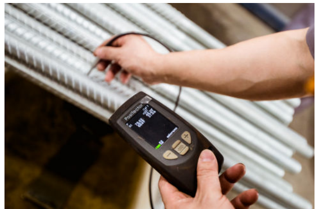
Control of coating thickness
